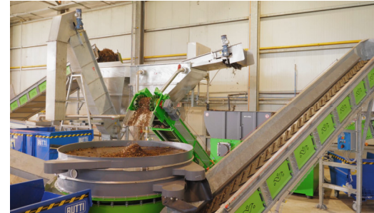
The biomass is cleaned, shredded and screened before entering the reactor
