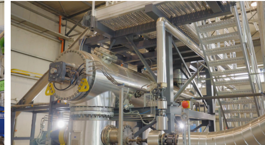
The reactor is continuously fed with biomass and injected with high-pressure saturated steam, operating at around 16 bars
